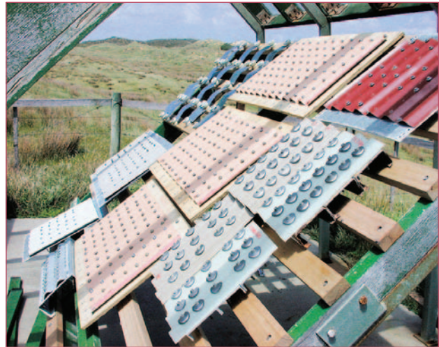
Above: Covered (unwashed) real-world test panel in marine environment.
