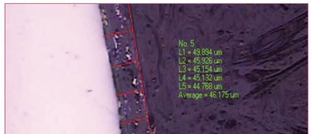
Above: Coating thickness.
